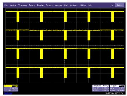
7. To display an individual segment separately from the main channel display, select Math, Math Setup from the menu bar, and choose a math trace to define as a Segment (in this case, we chose to define F4 as a Segment). As a source, use the channel that your CAN data was acquired on (in this case Channel 1). To display the trace, check the TRACE ON checkbox. To select the segment to view, touch the Select tab and select a segment using the pop-up keypad or the front panel adjust knob.
