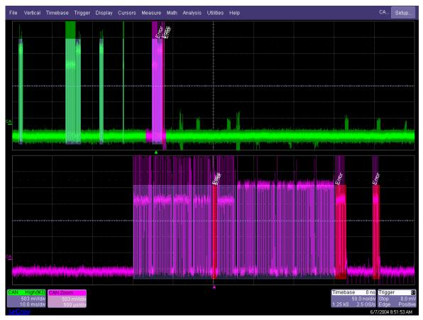
The CAN Zoom trace (light magenta) and the CAN Trace (green) are both displayed. The CAN Zoom trace is zoomed by a factor of 20 (the CAN Trace has a horizontal scale of 10 ms/div and the CAN Zoom trace has a horizontal scale of 500us/div). You can see the light magenta highlight on the green CAN Trace showing the position of the CAN Zoom.
